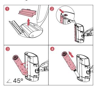
3 Insert a new cleaning roller onto the motor, push and fix it into the cleaning head till the lateral button in place.
