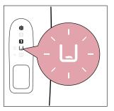
2 The tank full indicator starts flashing and the appliance stops operating when the dirty water tank is full. Empty the dirty water tank (please refer to 4.4 Emptying the Dirty Water Tank) and re-start the
