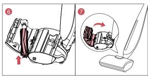
Note: The maximum open angle of the drive motor is 30°. Please operate it carefully.
