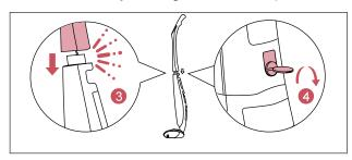
9 Insert the battery into battery compartment on the lower body and tighten the screw
