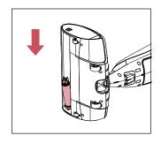
4 Insert the cleaning roller onto the motor (note: the maximum open angle of the drive motor is 45°), push and fix it into the cleaning head till the lateral button in place.
