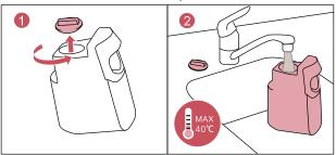
Note: If detergent is needed, only environmental friendly detergent authorized by HIZERO is allowed. First add the quantity of detergent indicated on the bottle packing and then fill the clean water tank with water.
