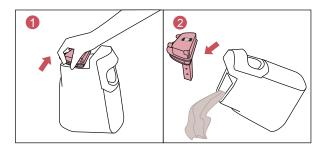
3 Rinse the empty dirty water tank and its cap under the tap, wipe dry the metal sensor plate. Then place the tank back into the appliance until you hear a click. To prevent the appliance from toppling over, hold it upright with one hand and place the dirty water tank with your other hand.
