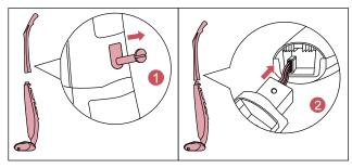
Note: Please flip to the other side of cable and try to connect again if the snap joint doesn't fit.
