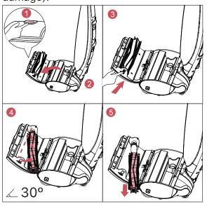
3 Insert a new brush roller, close the cover after it is well assembled.
